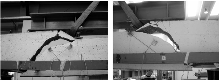
Figure 4.36: Crack patterns at failure for beam HSC-PC.
