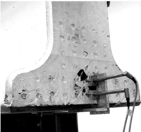
Figure 3.14: The instrumentation for measuring the cable movement.
