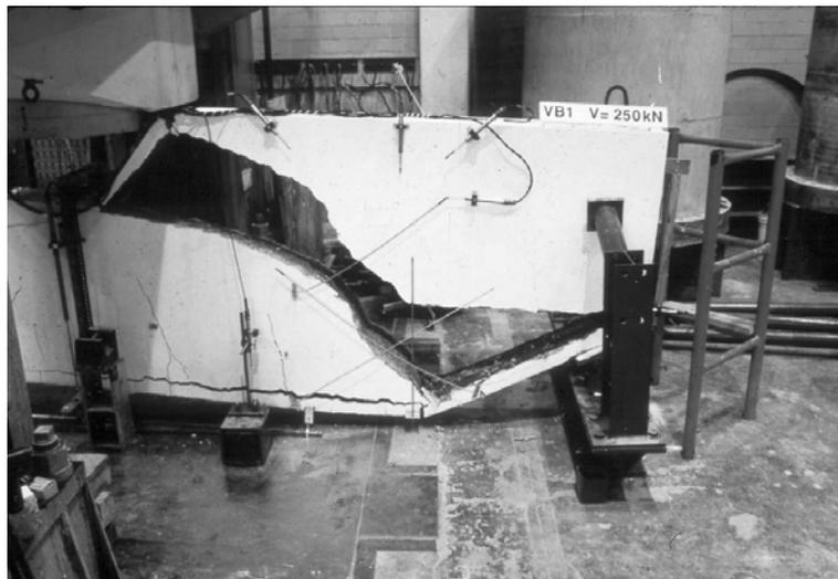
Figure 2.59: Shear failure of a deep beam tested at the University of Toronto.
