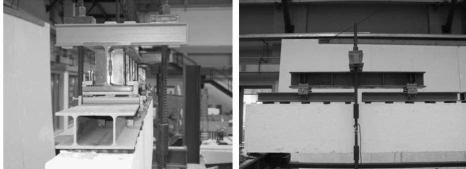
Figure 4.10: Loading system for the representation of a UDL.
