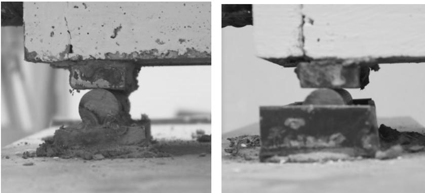
Figure 4.3: Pin and supports restraints, with the support steel plate connected to the specimen through a thin layer of high strength mortar.
