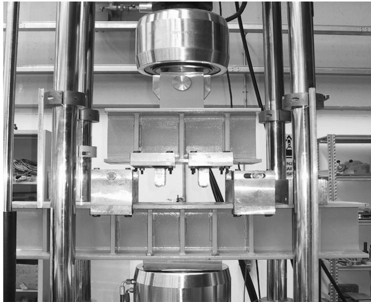
Figure 5.2: Top and bottom steel loading frame for performing four point bending test.
