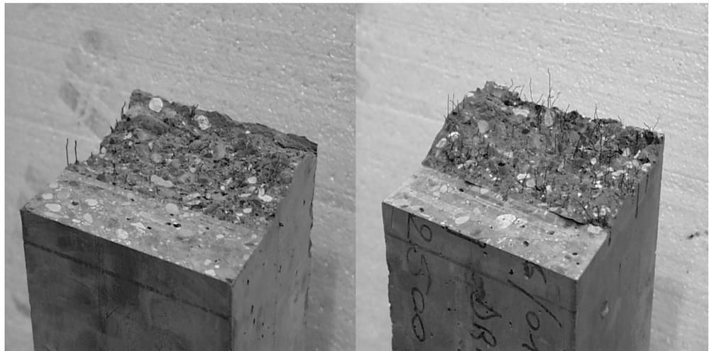
Figure 5.5: Ligament area of two different kinds of concrete mixtures after completion of test.
