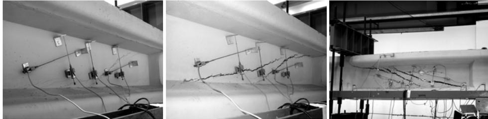
Figure 3.31: Crack formation and development, tests DZ, I-Beam 5 and I-Beam 6.
