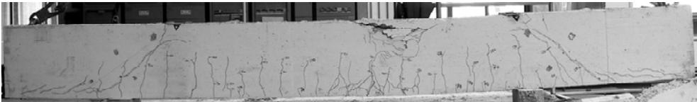
Figure 4.44: Comparison of final crack patterns, NSC1 series.
