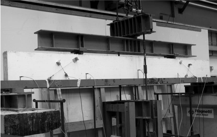
Figure 4.14: Picture of a specimen ready for testing. Note the potentiometric instruments measuring crack widths and strut displacements.
