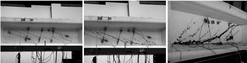
*Figure 3.28: Crack pattern evolution in TZ zone of the four beams.*
