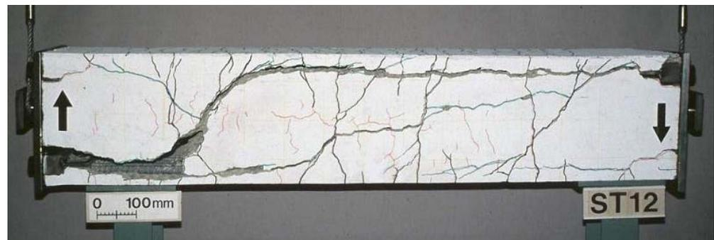
Figure 2.63: Typical crack pattern of a member without transverse reinforcement subjected to Axial tension and Shear.
