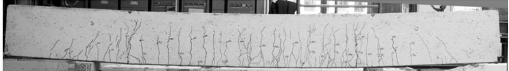
Figure 4.45: Comparison of final crack patterns, HSC series.
